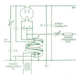
Fig. 2-With a grounded-plate amplifier, the stray plate-to-ground capacitance is in parallel with the grounding condenser, and is thus of no importance
