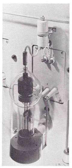
Saturated toroidal transformer — heart of arc-back indicator circuit — shown above mercury vapor tube.
