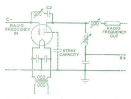
Fig. 1—The usual form of radio amplifier has a grounded filament and a plate at the radio-frequency potential
