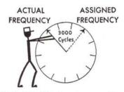
**ZERO HOUR:** Starting up after a shutdown, transmitter may be 3000 cycles above or below assigned frequency. **Frequency Watchman** goes to work.
