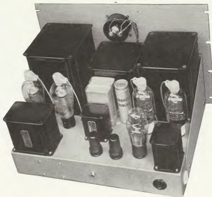
TOP VIEW SPEECH AMPLIFIER, MODULATOR AND HIGH VOLTAGE POWER SUPPLY
