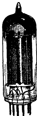
Rectifier valve or tube, giving full-wave rectification.
