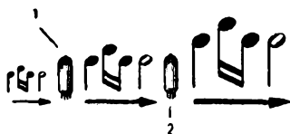
1 = 1st tube. 2 = 2nd tube. By means of these two tubes a double amplification will take place.
