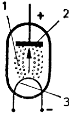
1 = flow of electrons. 2 = anode. 3 = cathode.
