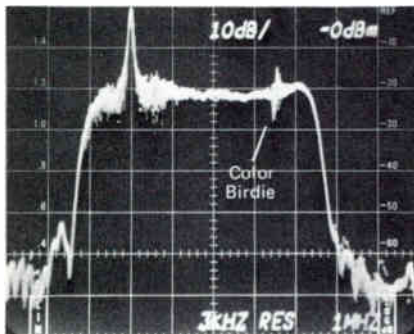
Figure 12. Low Level Sideband Response Using 3 kHz Resolution Bandwidth
