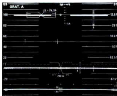
1. 60 Hz modified square wave used in testing for field time distortions.
