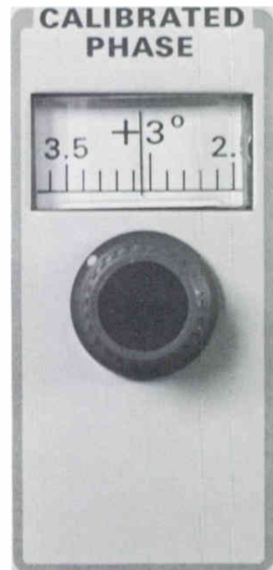
5. The CALIBRATED PHASE control is then adjusted to overlay the step being measured. The CALIBRATED PHASE dial now indicates the differential phase present. This method allows differential phase distortion as small as 0.1° to be measured.
