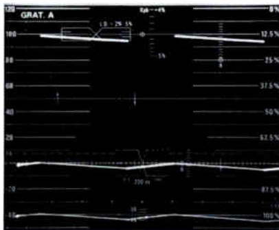
2. Field time distortion. Notice tilt in square wave. This check is made with the DC Restorer in the waveform monitor turned off.
