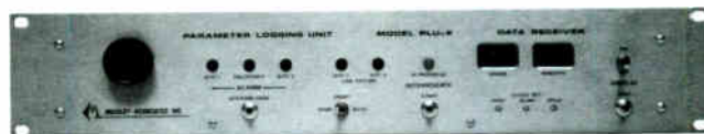
Model PLU-2 DATA RECEIVER. Time base is displayed on the front panel of the Data Receiver.
