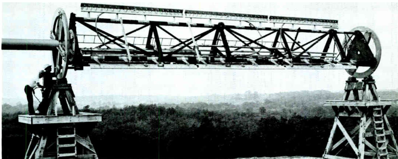
A three-layer Vee-Zee array undergoing pattern tests.
