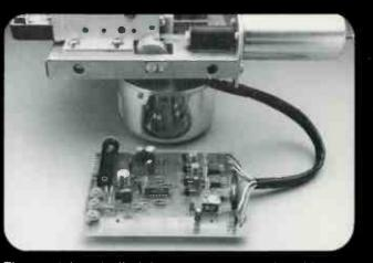
The crystal-controlled dc servo motor provides high timing accuracy, low heat generation and permits field speed changes.
