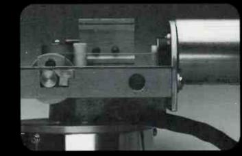
Pinch roller parallelism to the high-traction ceramic capstan is adjustable with the motor running.
