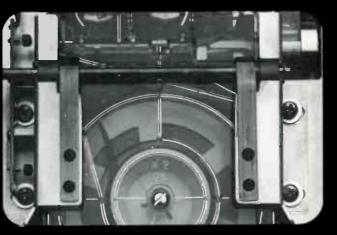
Carts are held by the edges to prevent distortion, with roller contact for easier insertion and withdrawal.
