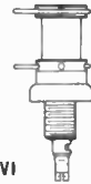
VI CLIP-TERMINAL TYPE Available with a or b slug-locking devices (see Fig. I)
