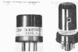
THERMALINE —Thermal Time Delay Relay. SPST NO or NC. 3 amp contact rating. Delays from 1/4 sec. to 3 minutes. Voltages up to 230 volts, A.C. or D.C. Details in Bulletin #60.
