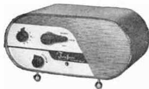
FIM-12, INTERMIX — $44.95. A deluxe twelve station intermix master which can be used in any combination of masters and/or remotes. Master has 3 position Talk-Listen-Dictate switch. Use in conjunction with two types of remotes: FC-6 which can selectively call any one of six masters, and FC which can call only one master. Weight: 4 lbs.
