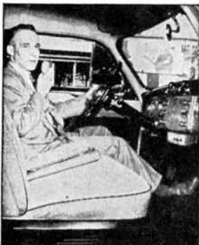
Illustrates Under-Dash Mounting for ATR Models RME and RMF. See Page 942 for available accessories.
