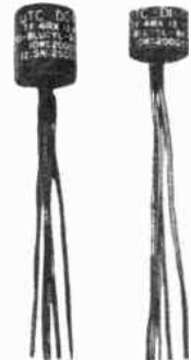
TRANSFORMERS PICTURED ACTUAL SIZE DO-T: 1/16 Dia. x 1/2", 1/10 OZ.; DI-T: 1/16 Dia. x 1/4", 1/20 OZ.
