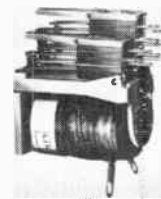
GT —Telephone Type Relay up to 6PDT in D.C. 4PDT in A.C. 5 amp contact rating. Voltages up to 110 volts, A.C. or D.C. Details in Bulletin #70.
