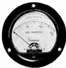
MODELS 25, 35, 45, 55 3 1/2" ROUND CASE—OPEN FACE STYLE. Flange diameter, 3 1/2"; depth overall, 2 1/4"; body diameter, 2 3/4"; scale length, 2 9/16". Bakelite case.
