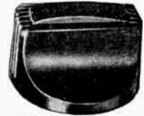
Cat. No. S-453-1 Walnut and black. No brass insert. Molded hole to fit standard \frac{1}{4} " shaft with one set screw. Diam. 1\frac{1}{8} " , ht. \frac{3}{8} " .
