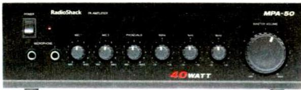
**40-watt PA amplifier with 3-band equalizer, mixer**
