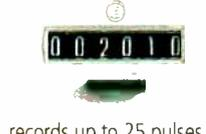
**Electromechanical counter.** Can count up to 999,999, advanced by external 12VDC pulse. Mechanical pushbutton reset. Accepts and accurately records up to 25 pulses per second.
