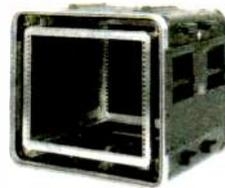
For the protection of the most delicate equipment against shock. This rack case has shock absorber coils at each of the eight corners to control damaging effects. The 20" rack depth allows for airflow around the frame. ATA approved.
