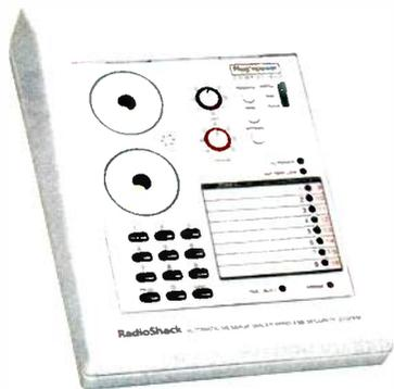
System includes controller console with auto dialer, motion detector, two door/window sensors, lamp module and handheld/keychain remote
