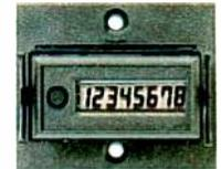
**Self-powered 8-digit totalizing counter.** 7mm high-contrast LCD. Self-powered for 10 years. Sealed to NEAMA 4. Front-panel reset pushbutton which can be disabled. Bezel and rear mounting clips supplied. External connection by standard plug or connector. 24x48 DIN standard case.
