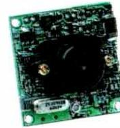
line-level video with excellent 380-line resolution and 1 lux low-light sensitivity. Requires 12VDC at 100mA. **980-0984** ..... 79.99
