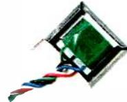
**1:1 isolation transformer.** For phone-line interconnects, coupling. 600-900 ohms. 300Hz to 5kHz response. 100-megohm insulation resistance at 250VDC. **273-1374**..... **3.99**
