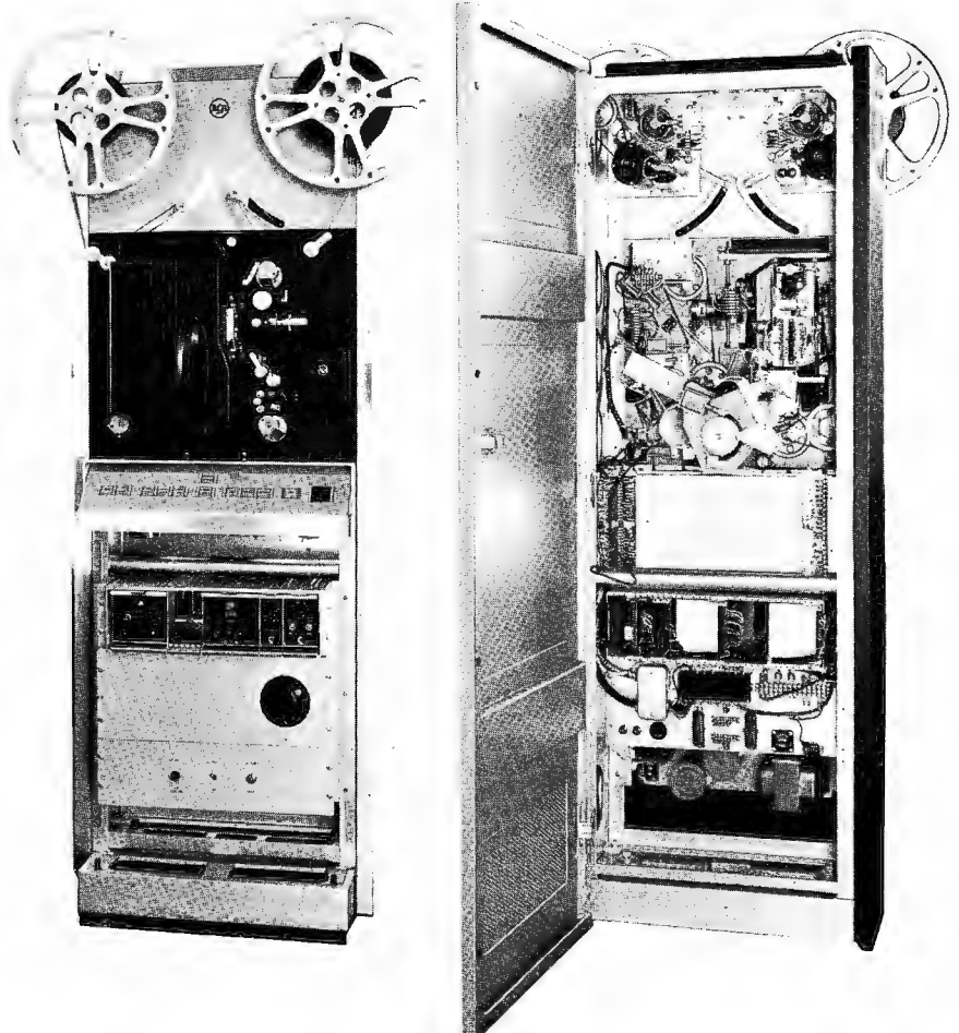
(Right) full length rear door (also removable) provides complete accessibility for inspection or service.
