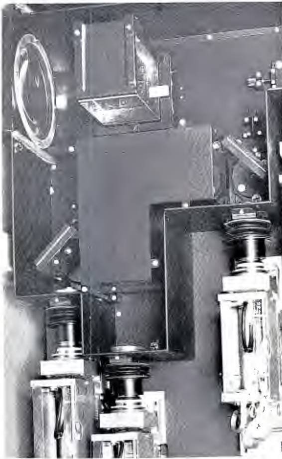
SEALED PRISM DICHOICS eliminate secondary reflections — are maintenance-free.
