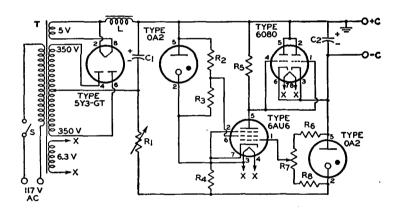
$C_1{=}20~\mu f,$  electrolytic, 450 v.  $C_2{=}20~\mu f,$  electrolytic, 150 v. L=8 henries, 50 ma, choke  $R_1{=}Current$  Balance Control, 5000 ohms, 25 watts, wirewound (Adjust for 60 volts across  $R_4)$
