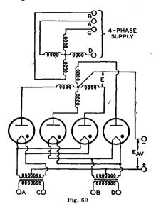
the use of in-phase filament and anode voltages may result in extremely short tube life.
