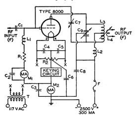
C<sub>1</sub>=0.0005  $\mu$ f, mica, 1500 v. C<sub>2</sub> C<sub>3</sub> C<sub>4</sub> C<sub>5</sub>=0.002  $\mu$ f, mica, 600 v. C<sub>5</sub> C<sub>8</sub>=0.002  $\mu$ f, mica, 5000 v. C<sub>7</sub>=5-10  $\mu$  $\mu$ f, neutralizing capacitor, air gap 0.3 inch min.
