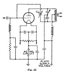
Consequently, C<sub>n</sub> is usually made adjustable over a small range on either side of the theoretical value.
