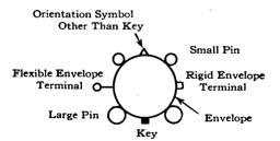
• = Gas-Type Tube BC = Base Sleeve G = Grid
