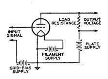
choice of operating conditions. For symmetrical driving voltages, the dc plate current remains substantially constant at the quiescent (zero-signal) value.
