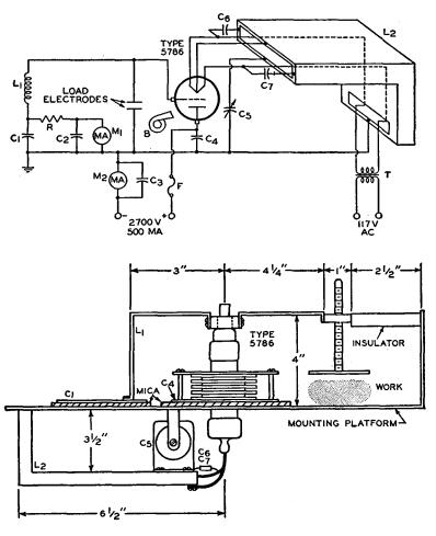
C<sub>1</sub>=250 μμf, mica 0.005 inch thick, 3 inches x 3¾ inches copper plate, held to mounting platform by insulated pressure clamps
