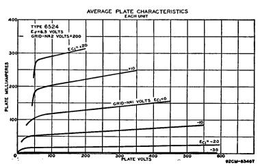
desired operating plate current after initial tuning adjustments are completed. Grid-No.2 voltage must not exceed 400 volts under key-up conditions.
