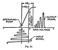
even-harmonic distortion and, consequently, requires the use of a push-pull circuit when used in audio or video service. The bias is adjusted so that the operating point is in the lower portion of the linear region of the characteristic. Because of the relatively small quiescent plate current, the tube can be operated at a higher plate voltage than would be permissible under class A conditions, and can thus deliver a higher maximum power output.
