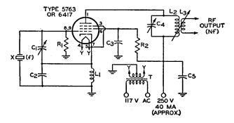
$C_1$ =3-35  $\mu\mu f$ , air trimmer  $C_2$ =200  $\mu\mu f$ , silver mica, 500 v.  $C_3$   $C_5$ =0.01  $\mu f$ , disk ceramic, 600 v.
