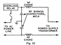
transformers having electrostatic shields between primary and secondary windings. Low-pass filters of the type shown in Fig. 53 are also useful. The bypass capacitors used in such filters must have a voltage rating at least equal to the peak voltage developed across each half of the transformer secondary (approximately 1.4 times the rms voltage).
