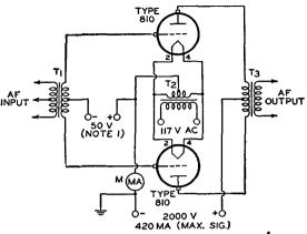
M=Milliammeter, 0-500 ma, dc T<sub>1</sub>=Driver Transformer, plateto-plate impedance 1500 ohms, turns ratio of total primary to one-half secondary 1.5 to 1 (Note 2) T<sub>2</sub>=Filament transformer, 10 v., 9 amp, center-tapped T<sub>3</sub>=Modulation transformer, load impedance 11000 ohms plate-to-plate; turns ratio depends on modulating impedance of modulated stage
