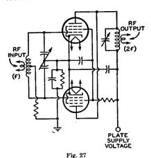
Additional information on the characteristics of frequency multipliers and the efficiencies obtainable for various degrees of multiplication is given in the Power-Tube Circuit-Design Considerations Section.
