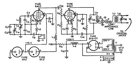
C<sub>1</sub>=15 μμf, ceramic, zero temperature coefficient C<sub>2</sub>=100 μμf, ceramic, negative temperature coefficient 750 PPM
