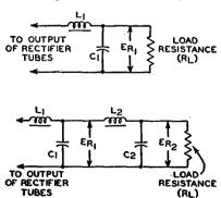
the desired filtering, serious instability may result if the combination selected is resonant at or near the ripple frequency. The inductance of  $L_2$ , therefore,
