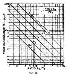
When the required tank-circuit capacitance is known, the tank inductance required for resonance at the desired frequency can be determined by substitution of the value of C in Equation (1). Approximate winding data for singlelayer coils, such as that shown in Fig. 37, suitable for use in amateur transmitters can then be obtained from the following formula:
