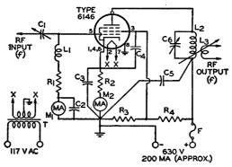
C<sub>1</sub>=4-50  $\mu\mu$ f, trimmer, air gap 0.015 inch C<sub>2</sub> C<sub>3</sub> C<sub>4</sub>=0.01, disk ceramic, 600 v. C<sub>5</sub>=0.005  $\mu$ f, mica, 1500 v. C<sub>5</sub>=2  $\mu\mu$ f per meter (approx-
