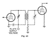
coupling between the plate and grid windings may be fixed or adjustable. Adjustable coupling provides a convenient means for controlling loading and excitation. The grid winding may be either tuned or untuned. Although the tuned type provides maximum efficiency, the additional control complicates tuning and is rather critical of adjustment.
