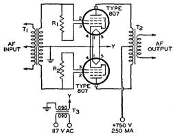
R<sub>1</sub> R<sub>2</sub>=20000 ohms, 1 watt, carbon
