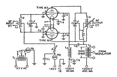
$C_1$ =0.005  $\mu$ f, mica, 600 v.  $C_2$ =2  $\mu$  $\mu$ f per meter per section (approximate value for resonance at frequency f), air gap 0.030 inch min.  $C_3$   $C_4$ =0.002  $\mu$ f, mica, 5000 v.  $C_5$   $C_6$ =0.003  $\mu$ f, mica, 5000 v.  $C_7$ =1.5  $\mu$  $\mu$ f per meter per section (approximate value for resonance)
