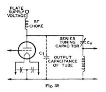
(4) Employ a "series-tuned" tank circuit of the type shown in Fig. 38, in which the variable capacitance  $C_v$  is several times larger than the tube capacitance  $C_t$ .
