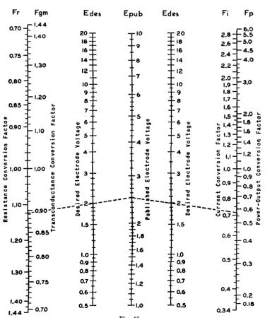
a tube is changed, for example in the calculation of operating conditions for a multigrid tube operated at a grid-No.2 voltage for which curve families are not available, the nomograph is used twice. The procedure is shown in the following example:
