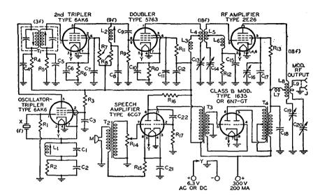
$C_1=150 \mu\mu f$ , mica, 600 v.  $C_2 C_5 C_{22}=0.005 \mu f$ , disk
