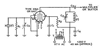
C<sub>1</sub> C<sub>4</sub>=0.005  $\mu$ f, mica, 600 v. C<sub>2</sub>=1.0  $\mu$  $\mu$ f per meter (approximate value for resonance at frequency f), variable, air gap 0.015 inch
