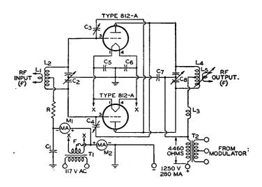
C<sub>1</sub> C<sub>5</sub> C<sub>6</sub>=0.005  $\mu$ f, mica, 600 v. C<sub>2</sub>=2  $\mu$ mf per meter per section (approximate value for resonance at frequency f), air gap 0.026 inch, min. C<sub>5</sub> C<sub>4</sub>=4-10  $\mu$ mf neutralizing capacitor, Hammarlund NC-75 or equivalent C<sub>7</sub>=0.002  $\mu$ f, mica, 5000 v.
