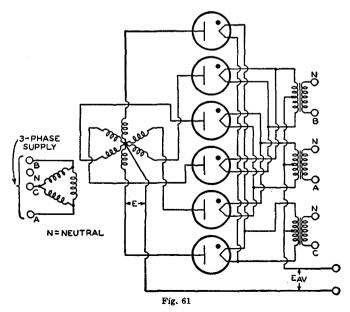
by supplying the filament of each rectifier tube with voltage out of phase with its anode voltage. Although the ideal phase relationship between filamentsupply voltage and anode voltage is 90 degrees (true "Quadrature"), substantial benefits are also realized at phase angles of 60 or 120 degrees, which are readily obtainable in three-phase and six-phase rectifier circuits.
