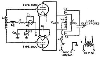
$C_1$   $C_2$   $C_3$ =0.005  $\mu$ f, mica, 600 v.  $C_4$ =2 plates 3/32-inch aluminum, 5 inches x 7 inches spaced 7/8 inch C<sub>6</sub>=50 μμf, max., depends on
