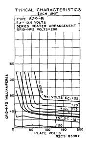
In ICAS applications, at frequencies less than 20 Mc, where the duty factor does not exceed 0.2, maximum "on" period does not exceed 30 seconds, and average modulation factor does not exceed 0.25, maximum grid-No.2 input of 12 watts is permitted.
