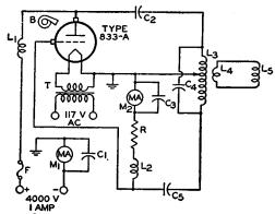
C<sub>1</sub> C<sub>3</sub>=0.01  $\mu$ f, mica, 600 v. C<sub>2</sub> C<sub>5</sub>=0.1  $\mu$ f, paper, 5000 v., 0.6 amp rms min.  $C_4=0.002 \mu f$ , mica, 8000 volts min., 15 amp rms
