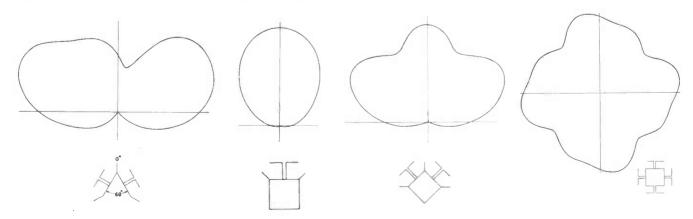
formance of the Super-Gain antenna is independent of the supporting tower construction. The cross-section of the tower is determined by the operating frequency; however, the tower can be either rectangular or triangular in shape.
