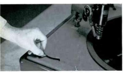
A SINGLE "OFF-ON" lever controls both synchronous turntable drive motors. In "OFF" position, a brake brings turntable to quick stop.
