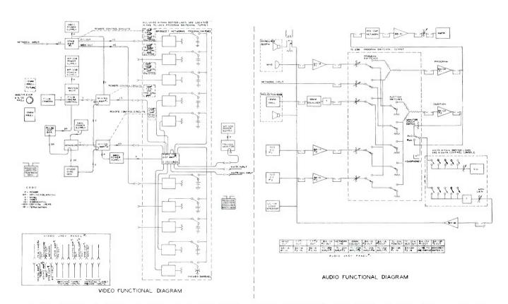
Block diagram of typical installation using five program sources. Amplifying equipment is shown with power supplies indicated where needed.
