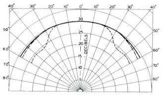
DIRECTIONAL CHARACTERISTICS OF A TYPICAL LC-1A SPEAKER IN CABINET
