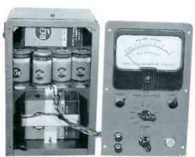
Removable panel provides easy access to batteries
