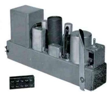
is shock mounted to prevent microphonics. The circuit is conventional with unloaded transformer input, resistance-capacitance coupling between stages and transformer output. The distortion and hum level has been reduced to a very low value through proper circuit design and through the use of stabilized feedback. Cross talk between units is -75 dbm, 50 to 15,000 cycles when mounted side by side and operated from the BX-1D Power Supply.
