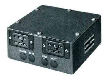
ing the Cathode Ray Oscilloscope driving pulse. This terminal provides an auxiliary method of drive, since the driving pulse is carried by other means in normal television station operation.
