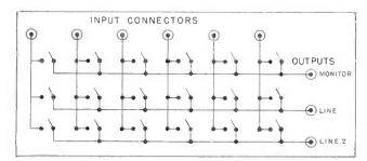
way, a local monitor connection with a capacity up to 200 mmf can be used. In cases where the monitor capacity is less, fixed padding condensors can be paralleled with the output to bring the total up to 200 mmf. This is done to prevent disturbing the response of the monitoring network.
