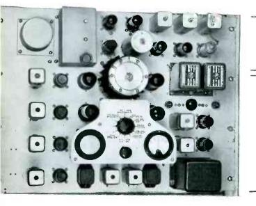
BASIC CIRCUITS are mounted on this part of the exciter panel. They include two audio modulators, an FM oscillator, and three frequency multiplying stages (see diagram above).
