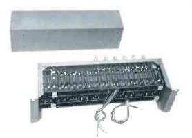
View of Sync Generator Delay Panel shown with protective cover removed
