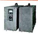
RCA Field Synchronizing Generator IG-10A. Produces timing pulses for TV field equipment. Unit No. 1 includes pulse-forming circuits, frequency-control circuits, and power supply. Unit No. 2 includes the pulseshaping and output circuits.
