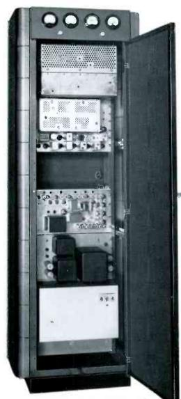
Eighty-four inch cabinet with door open showing from top to bottom: CT-6C Power Ampli-fier, Exciter, CR-9A Receiver, and Transmitter Power Supply.
