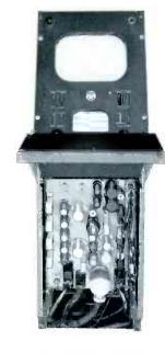
Studio Camera Control Unit consisting of TM-5A Monitor and Camera Control Chassis (M1-26055) mounted in console housing (MI-26266B)
