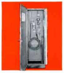
L-F ANTENNA DIPLEXER (left) AND THE VESTIGIAL SIDE-BAND FILTER (right). Diplexer makes it practical to use one antenna for picture-and-sound signals. Side-band filter partially suppresses one sideband. No adjustments required.
