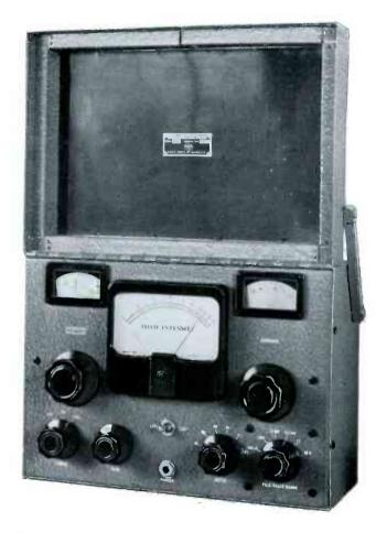
The direct reading feature of the WX-2C simplifies field intensity measurements and eliminates the needs of the usual attenuator readings, meter readings and multiplication factors. A wide sensitivity range, 10 volts per meter to 10 microvolts per meter, permits maximum flexibility of operation within the range of 540 to 1600 kc.
