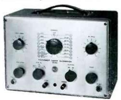
features which mean speed, accuracy and reliability...if center frequency 8.3 to 10.8-Mc...adjustable if sweep width...facilities for external frequency modulation...rf range continuously variable from 85 to 110-Mc...includes step and fine attenuators...a 'scope phase control permits centering of sweep patterns. Provides the signals you need for fast, accurate FM alignment Shipping weight, 17 lbs.
