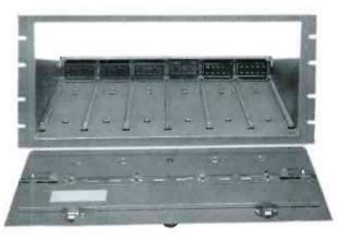
Panel removed showing guide bars and receptacles
