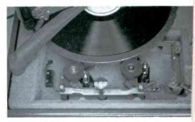
OH-78 RPM—In "ON" position, the brake shop moves away from turntable rim and rim and rubber iclers are now in active contact with drive wheel and turntable rim.
