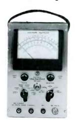
Portable electronic voltmeter-ohmmeter and ammeter combination for mobile, industrial or rural use. Works anywhere without a-c power source, thereby extending famous VoltOhmyst features to places remote from power lines. Neon panel lamp lights when battery is used. Unusually long battery life with normal use.
