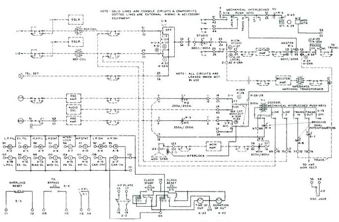
Simplified Schematic Diagram of the MI-11621 Console
