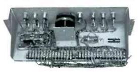
OVER). Associated tally lights, slide projector on-off switch, slide projector fader control for controlling lamp brightness and tally light are also provided. All circuits and push-button contacts terminate in terminal strips mounted at the rear of the changeover panel.
