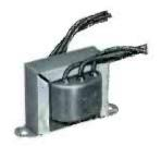
This transformer is ideal for operating a number of medium power speakers with a voice coil having 6 or 2 ohms impedance. The primary winding has three taps for 4000, 8000 and 16,000 ohms. It is designed for bracket mounting and has 10"
