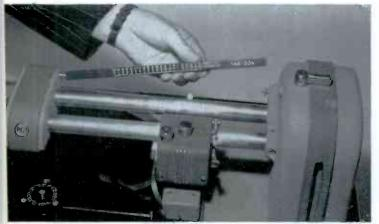
CALIBRATED TIME SCALES for 96, 104, 112, 120, 128, 136, 144 and 152 ("inside-out," "outside-in," at 33\% or 78 rpm are provided. Here, proper scale to agree with "pitch" setting is inserted.
