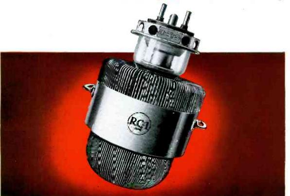
The revolutionary, new power triode RCA-5671. This tube takes about one third the filament power of conventiona triodes used in the older transmitters. It reduces hum modulation below FCC requirements—even without r-f feedback
