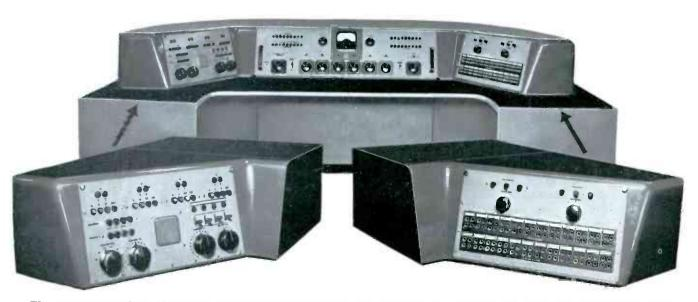
The arrangement above shows how special matching consoles are designed for desk-top use with any standard 76-series consolette. Such consoles may contain special talkback facilities, order wire ringdown circuits, monitor controls and signal lights. Jack panels may be included, if desired, for use with the 76 consolette. In addition to the special end cabinets shown here, "straight" type cabinets to match 76-series consolettes are also available.
