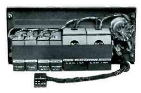
Rear view of Battery Cover showing batteries mounted in place
