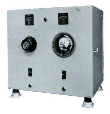
stand located near the wall of the mobile unit directly behind one of the operators' seats. Heavy shock mounts are provided with the cabinet.
