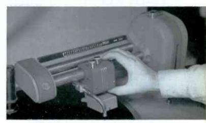
**CARRIAGE LEVER** is being pressed to allow movement of recorder-head horizontally over the record to desired "cutting" position.
