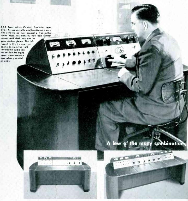
BTC-IA Control Console—with transmitter-control turret, audio control turret, and blank turret for additional facilities such as special meters, jack fields, ringdown, etc. Front panels are bottom-hinged. Rear covers are removable.
