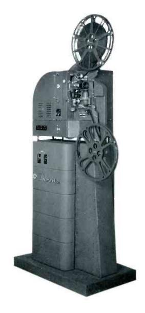
The film feed arrangement of the TP-16B is identical to that of the standard projector with the exception that the pull-down claw works at a greater speed. Film is fed from the upper reel under a large sixteen-tooth feed sprocket and through the precision made film gate. Light, controlled by a rotating shutter, is projected through the film at this point. The film is pulled down through the gate, a single frame at a time, by the pull-down claw just below the gate.
