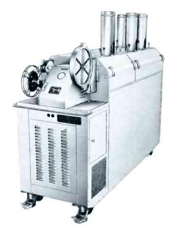
solution level maintained in the various tanks by overflow drains at the top. This overflow is piped to a single drain line at the rear of the machine. Processing speeds for reversal film are dependent upon the manufacturer's specifications and type used. Speeds of 18 to 35 feet per minute are possible, dependent on the film type.
