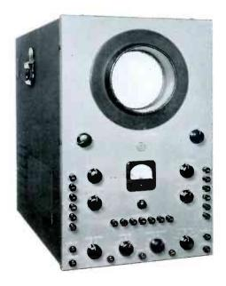
It features triggered sweep and blanking circuits that permit the observation and photographic recording of one-time, highspeed transients. This oscilloscope also shows a-c and d-c simultaneously, providing more information than can be obtained from a simple stroboscope. The 5-inch C-R tube can be readily interchanged from the front with a tube of other persistence characteristics.
