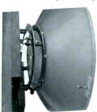
reflector, may be adjusted in both horizontal and vertical planes by means of hinged links and locking bolts. Adjustments provided on the gimbal ring permit a  $\pm 71/2$  degree horizontal and vertical movement.
