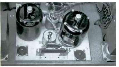
**TWO SYNCHRONOUS MOTORS** hysteresis type, are coupled to wheels which rim-drive the turntable through sturdy, rubber-idler rollers.
