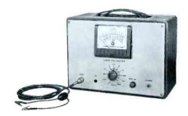
Input Resistance and Capacitance\_\_\_\_1 megohm shunted by less than 25 unf
