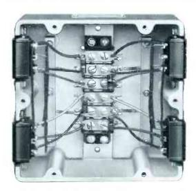
Pulse Distribution Box with cover removed
