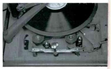
AJ-33<sup>1/2</sup> RPM—With speed change knob "UP," subberidlers are moved vertically to low-speed position of drive wheel that "lo- and hi-speed" shoulders at different diameters).
