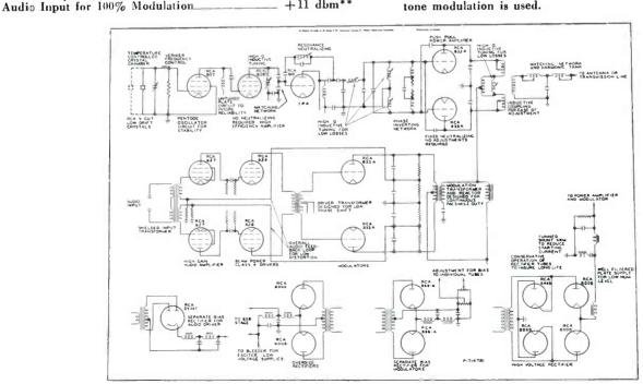
Simplified Schematic Diagram of BTA-1L
