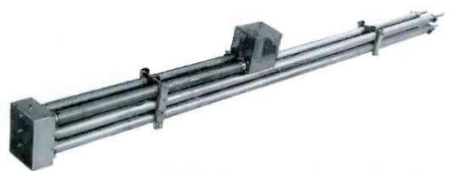
The Video Unit contains the detector, amplifier and power supply. This unit also contains a tuned vibrating relay which can be operated when zero output level indications are required for measuring percentage modulation of the visual transmitter.
