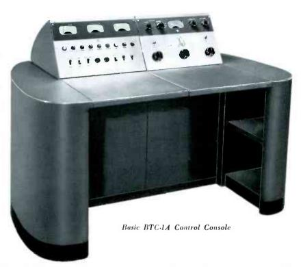
different inputs—one microphone-oscillator or remote, two different lines, and two separate turntables—with three high-quality mixers and associated transfer keys. A microphone key cuts off the signal to the monitor amplifier—and prevents feedback when the microphone is in use. A line transfer key removes equalization and connects the telephone to the particular line not in use.
