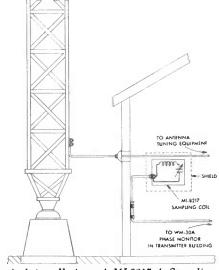
Typical installation of MI-8217-A Sampling Coil
