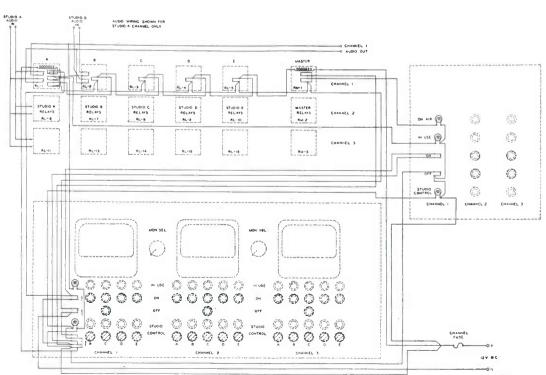
Schematic diagram of BCS-1A Switching System
