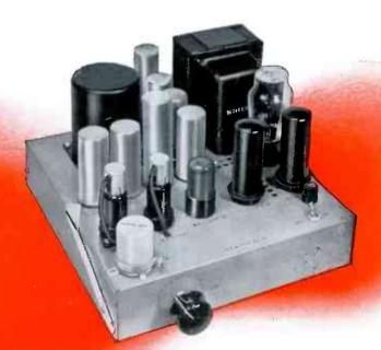
Monitoring Amplifier (Type BA-14A)—Designed for operation at microphone levels. High output of 12 watts is sufficient to drive several speakers or, in some applications, a recording head. Other uses include application as line amplifier for portable and mobile transmitters. High gain: 105 db. Low noise level: —20 db (with maximum gain); —40 db (with minimum gain). Low distortion: less than 3% at 12 watts. Frequency response: ±2 db, 30 to 15,000
