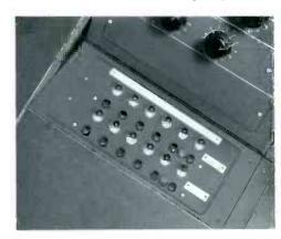
M1-26222 Master Control Panel shown mounted in sloping desk portion of TV console section.
