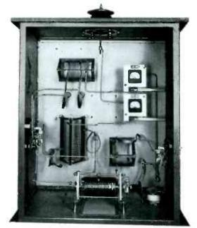
Interior view of a 5 KW line terminating unit mounted in a BPA-1A Housing
