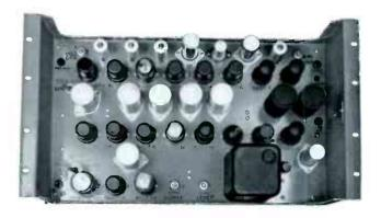
A two-position attenuator at the input accommodates a range of input signals from 0.25 volt to 15 volts, peak-to-peak. The output of the amplifier is designed to deliver the standard level of picture and blanking signal (1.5 volts, peak-to-peak) with a maximum sync of 1.5 volts peak-to-peak. The amount of sync can be adjusted independently to any value between 0 and 1.5 volts, peak-to-peak.
