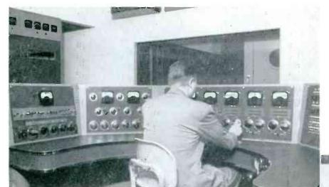
KOMO, Seattle. This master contro! console—with 9 deluxe audio equipment racks (at rear, not visible)—is one unit of KOMO's completely new and modern 7-studio system. It incorporates complete center panel switching for 10 studios and 6 outgoing channels (KOMO-AM, KOMO-FM, network plus 3 emergency).
