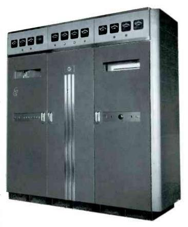
The power control circuits include both manual and automatic overload protection. When in the automatic position, a 3 shot recycling sequence is provided by the control "brain center" which automatically returns the transmitter to the air up to two times in case of repeated overloads. If such an overload condition still persists the transmitter is automatically shut down on the third overload.
