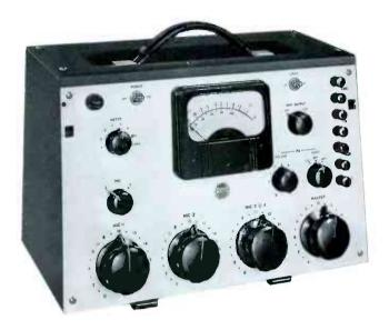
The steel case is ruggedly constructed with the front cover easily removed for quick operation. Accommodation for carrying spare tubes and fuses is provided within the case.
