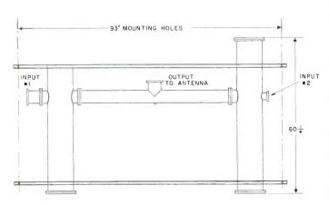
plicable to one input of the dual input filter. Thus a 10 kw filter can accommodate a maximum power of 20 kw, 10 kw on each input, and a 50 kw can handle a total input of 100 kw. Any power up to the rating can be used on either input of the filter.
