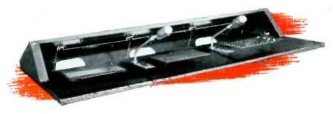
RCA Program Directors Console Type TC-5A. Television's most up-to-date directors' control. Includes large-size picture monitors for the studio outgoing line, for previewing, and for "on-the-air" monitoring. All switching under finger-tip control. Low height for full studio visibility. Recessed monitors for maximum image brightness in a fully-lighted control room.
