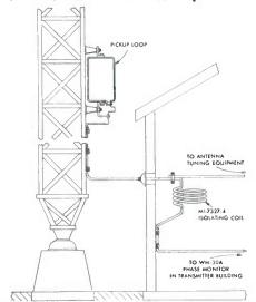
Typical installation of MI-8217-D Pickup Loop and MI-7327-4 Isolating Coil
