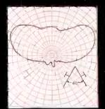
60° angle between dipoles 0° phasing between dipoles
