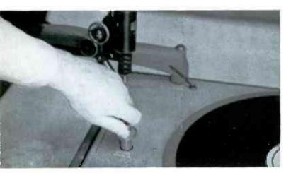
**SPEED-CHANGE** is simply accomplished by operating the control knob shown here. "UP" is  $33\frac{1}{3}$  RPM—"DOWN" is 78 RPM.
