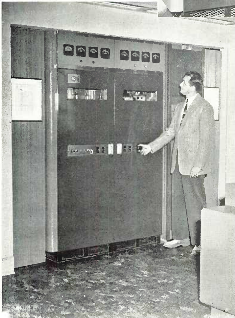
One kilowatt FM transmitter, Type BTF-1C, as installed at radio station WBRE-FM, Wilkes-Barre, Pa.
