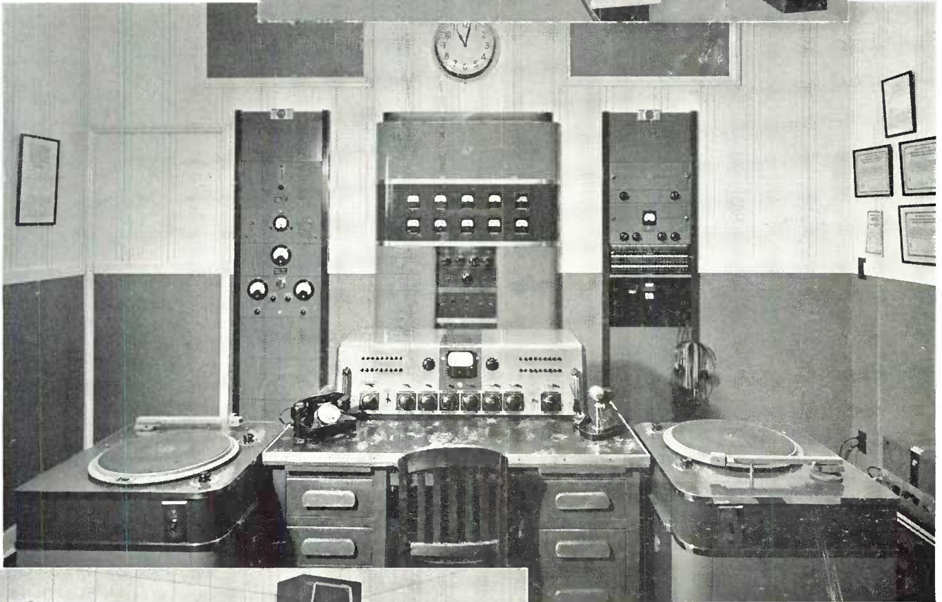
Control room at WMRN, Marion, Ohio, showing 250 watt transmitter, turntables, control console, and associated audio and test equipment.
