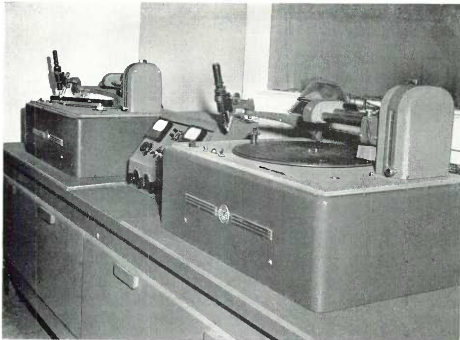
An ideal recording installation at KECA, Los Angeles, Calif., showing two of the four RCA 73-B Professional Recorders. Note the conveniently located overhead lighting, the large size suction duct, and relatively short length of hose for chip removal.
