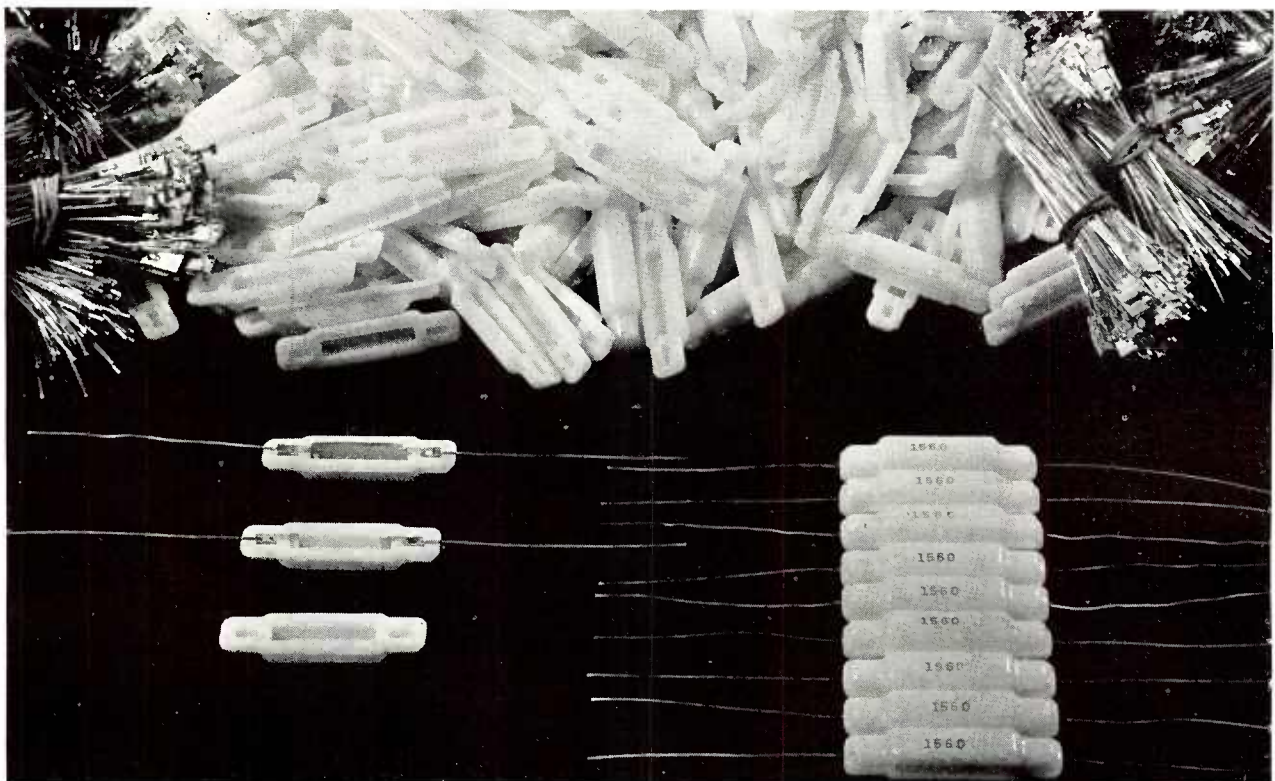
One of the Many Types of Crystals Developed by RCA for Special Applications.
