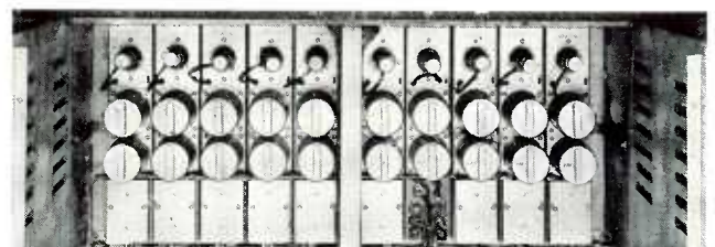
Ten RCA-85-B Preamplifiers mounted in CBS Type 2-A Studio Control Desk
