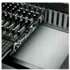
Two group output modules are offered: a basic group output module (WU-8107) comprised of a fader, LR send and pan, solo and group on switches and a return control; and a tape monitor group module (WU-8102) with all the features of the basic group module except for the channel on/off
