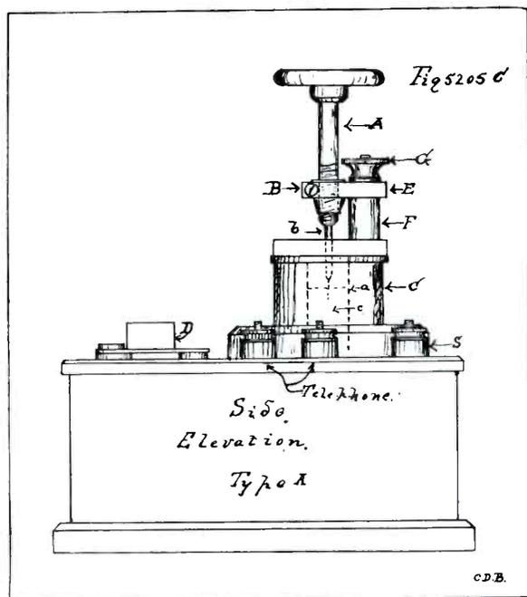
Figure 10 — Drawing of 3BV's electrolytic interrupter or "pulse modulator."
