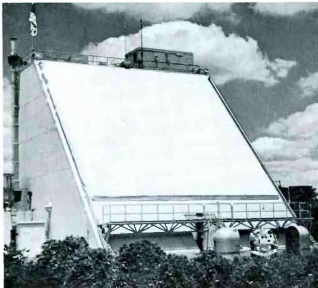
Figure 2B — Scale model of L-band ESAR radar shows equipment location. Air-conditioning of unit provides the constant temperature-humidity necessary to maintain phase control.
