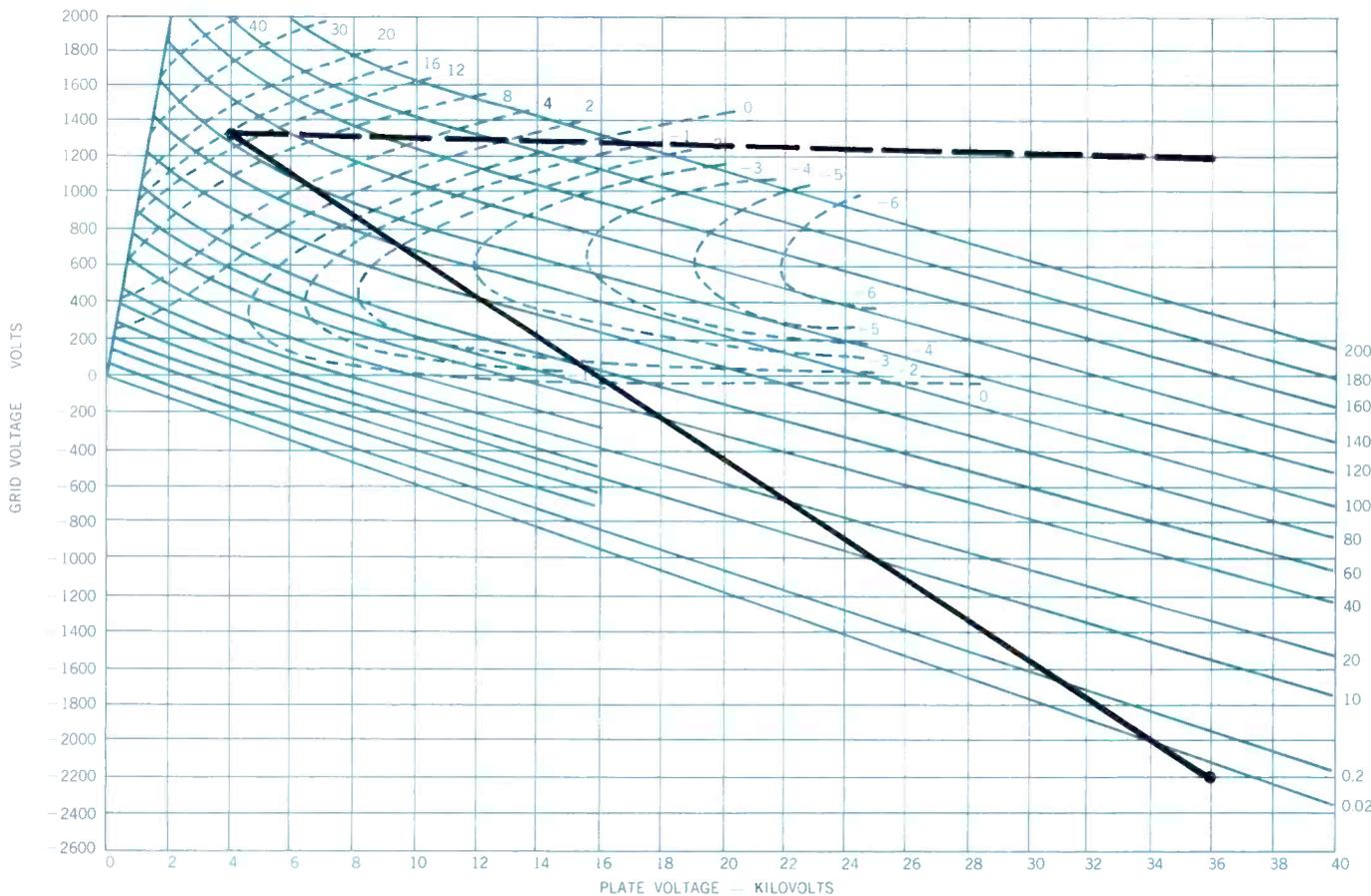
Figure 2 — ML-6696 Constant Current Characteristics showing normal load line as solid line, and load line when load arcs as dotted line.
