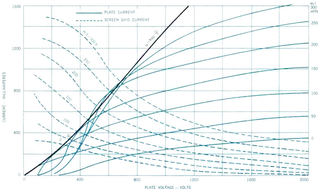
Figure 4 — Typical Constant Grid Voltage Characteristics. Line labelled  $i_b = K\epsilon p^{3/2}$  shows plate current drawn from virtual cathode formed between screen grid and plate.
