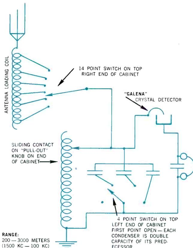
Figure 7 — Schematic drawing of the 3BV receiver.
