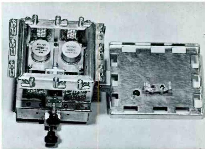
Figure 2 — Individual enclosures to permit maximum tube cooling are employed for the tuned line tripler, mixer and final amplifier stages. The final amplifier stage is illustrated.
