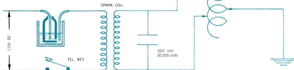
Figure 9 — Schematic drawing of the 3BV transmitter.
