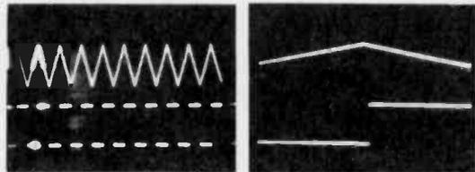
The delayed sweep takes the user selected portion of the waveform (intensified portion in the left picture) and magnifies it the desired number of times for closer examination (right picture).
