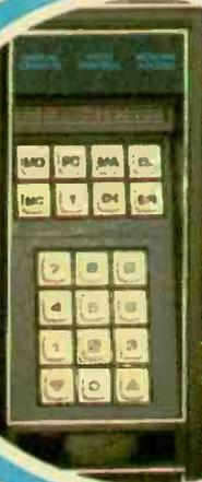
Eight programming pushbuttons let you sequence the GR-2001 to change channels and rotate your antenna (with optional GD-1184 Rotor) at times you preselect! Above the pushbuttons, backlit nomenclature shows the current operating mode of the programmer.
