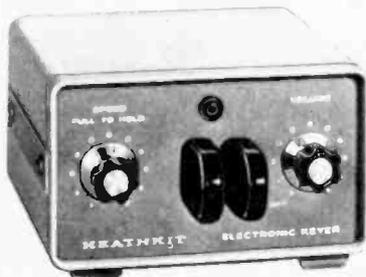
Your CW transmissions will be 100% copy with the HD-1410, because sending code is easy, whether you're operating base or portable. The dot and dash paddles travel and tension are easily adjustable. When the two paddles are treated as one, the HD-1410 operates like a single-paddle keyer with dot and dash memories, lmbic operation forms most characters with reduced wrist movement. Dots and dashes are self-completing and always in proper proportion.
