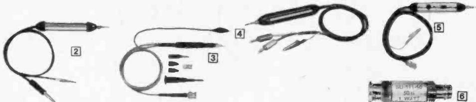
**3** Combination X1, X10 Scope Probe. DC to 15 MHz (X1) and DC to 80 MHz (X10) bandwidths. X10 rise-time. 3-position slide switch, 4.5' cable.
