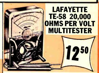
20,000 Ohms Per Volt DC-10,000 Ohms Per Volt AC
