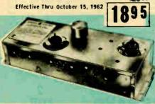
This adaptor is designed to operate in conjunction with FM tuners to provide two stereophonic audio channels. Completely self-contained and self-powered, the only required connections are those to the separate inputs of the stereo tuner. Frequency response: ± 3db 50 to 15,000 cycles. Hum and neise down 60 db. Mounting base is 10Lx21/4"W, with mounting holes spaced 21/4".
