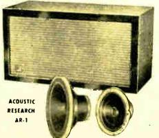
Bosed an new acaustic suspension" principle. Utilizes cobinets filled with Fibreglas, and with specially-constructed speaker-mechanism suspension plus air-tight cobinet in which campression of the oir by the speaker causes spring-like return at the speaker cone.
