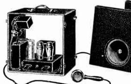
There are many uses or a reality portable public address system that a man can carry single-handed and set up in a short time. The new Lafayette Dual Speaker System ills the bill perfectly. Not only is it compact enough to carry in a train or in the runble seat of a car, but it also is a high quality dectrical instrument incorporating the newest developments in amplifier practice.
