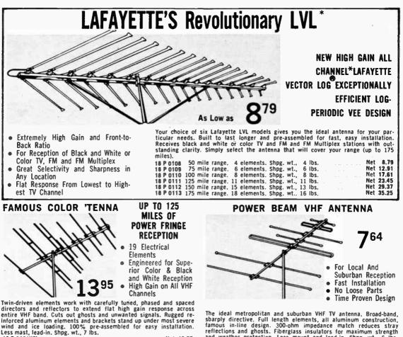
sarply directive. Full length elements, all aluminum construction, famous in-line design. 300-ohm impedance match reduces stray reflections and ghosts. Fiberglass insulators for maximum strength and weather protection. Less mount and lead-in. Shpg. wt., 6 bs. 18 P 0102WX Net 7.64
