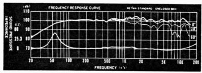
= 20 TO 20,000 CPS (40 TO 16,000 CPS ± 3 DB) = HIGH EFFICIENCY = HIGH EXCUR-SION WOOFER WITH UNIQUE "CONICAL STIFF-ENER" = HANDLES HEAVY BASS PASSAGES WITHOUT "DOUBLING"
