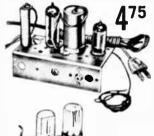
Have fun making announcements and broadcast-ing music through your own radio — with this broadcaster. Simply connect high impedance mic-rophone or phono pickup to broadcaster and tune in broadcaster and radio set. Pretuned to 1600 on radio dial but easily retuned. With 128E6 and 35W4 tubes, phono jack, 2 feet of antenna, sche-matic and line cord. Completely wired. Chassis size: 4X2". For 110-125V AC/DC operation. Shge. wt., 2 lbs. Yat P 1301 . Net 4.75 24 P 1301 Net 4.75
