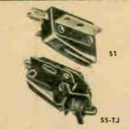
Wide range 50-15,000 cps ceramic cartridges unaffected by humidity and temperature. Feature high compliance and low distortion. .7V output. Replace crystal cartridges. Replaceable single sapphire stylus. Needle Pressure 8 grams. ½" mtg. centers. Type 51 also has additional holes for %" mtg. in 45 RPM changers. Type 53-2J replacement for Sonotone W7590.
