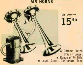
Model 32. Custom quality chromed trumpets with loud clear, piercing, continental tone. Range up to ½ mile. Ideal for use on trucks, sports cars, emergency vehicles, buses, boats, etc. Compressor pumps air to trumpets instantly when horn is pressed—there's no waiting for pressure to build up. Supplied with Town and Country Selector Switch which enables use of original horns for city driving, Comprete with: 2 horns (7" & 9"), compressor. fittings, horn relay,
