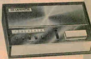
cuitry for "instant on" operation. Incorporates a balanced 40 ohm input and output circuit design. The advantages of this type of design is that the entire system when operating is virtually not susceptible to noise interference. Master unit has 5 individual station selector slide switches, 2 position press to talk—talk-took bar, and volume control. Remote unit has 2 position press to talk—talk look bar. Handsome walnut wood cabinet with brushed aluminum finish. Includes junction box for wiring.
