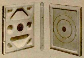
Lafayette "Poly-Planar" wafer-type component loudspeakers employ a lightweight acoustic panel supported by a frame of polystyrene plastic material to reproduce a range of frequencies from 40 cps to 20,000 cps. This material also permits the speakers to be made impervalues to extremes of temperature, humidity, shock, and vibration. There is also a minimum of piston motion resulting in low distortion and high electromagnetic efficiency.
