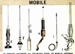
(E) FAMOUS LAFAYETTE ALL STAINLESS STEEL CB MOBILE ANTENNA Full quarter wave 102-inch stainless steel whip, heavy-duty chrome plated stainless steel spring and swivel ball jointed base designed for mounting on any surface. Base has lug terminals for 42 - 7002 cable assembly. Perfect for rear deck mobile mounting. Less cable. Imported. Shpg. wt., 4 lbs.
