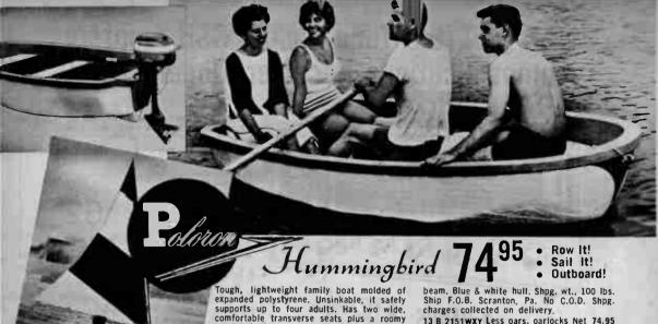
insulated storage compartment which dou-bles as an extra seat. Maintainance free solid one piece construction is unaffected by salt water. Weighing only 48 lbs, it can be easily transported on car roof—requires no docking facilities. Can be used with outboard motor up to 3.5 HP (below), oars, or optional sail kit, Length: 9 ft. 3 in. 52" 13 B 2151WXY Less oars, oarlocks Net 74.95
