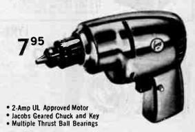
Lafayette's top drill value, 1/4" geared chuck drill rated at a full 2.0 amps, UL approved, 1/4" capacity in steel, 1/2" in hardwood, 1200 MPM speed under full load; 2000 RPM no load speed. Precision antifiction bearings, Automatic trigger switch, Specially designed gear train for maximum torque transfer, Mirror finish, Overall length 8". For 115 volts. AC/DC. Shpg. wt., 3 lbs.
