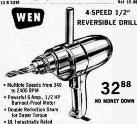
Model 950—A versatile, heavy duty ½" drill to handle big jobs—where great power is required. Quick, easy two-lever control of electronic and gear reduction speed changes permit efficient use of hole. All 4 speeds are reversible too with extra safety double switch. 6 amp. ½ horsepower motor, 120V AC/DC. 6 ft. 3-wire cord. UL and CSA approved. Size 11x8½x3½" (LHW). Die Cast aluminum housing, balanced for continuous operation. Shpg. wt., 9 lbs.
