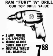
Lafayette's top drill value. ¼4" geared chuck drill rated at a full 2.0 amps. U/L approved. ¼4" capacity in steel, ½2" capac-ity in steel, ½2" capacity in hardwood. 1200 rpm speed under full load, 2000 rpm no load speed. Precision anti-friction bear-ings Automatic trigger switch. Specify de-signed gear train for maximum torque transfer. Overall length 8". For 115 volts, 25-60 cps AC. Shgg. wt., 4 ibs. HD-708 HD-708 Net 7.88 EL-109 50-ft., 3-wire Ext. Cord .. Net 3.51
