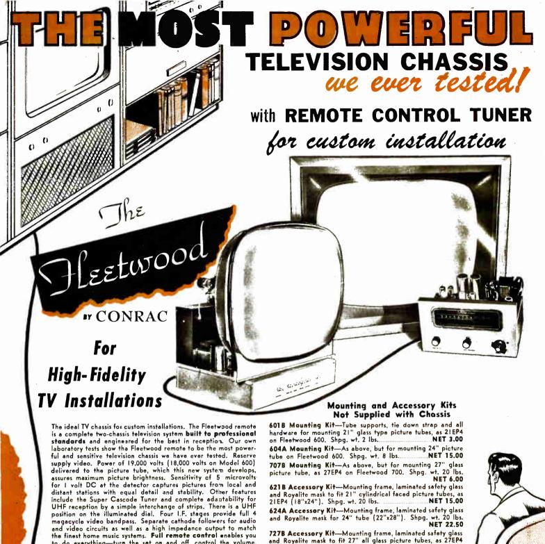
to do everything—turn the set on and off, control the volume, select your stations, adjust the contrast and fine tuning—without leaving your chair. Dimensions: Tuner chassis 7" H x 11½" W x 8½" D; Picture chassis (21" tube mounted) 21" H x 20¾" W x 23¼" D; Picture chassis (24" tube mounted) 30" H x 26" W x 25½" D; Picture chassis (27" tube mounted) 26" H x 25½" W x 231/4" D.
