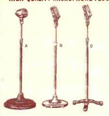
All adjustable smoothly and noiselessly, and provided with wear-ever, suregrip automatic friction clutch locks for firmly locking the stands at any desired height. The hard-ened fibre bush-ing in the clutch practically indestructible. 411 have tubing of heavy gauge metal, triple chrome plated. All have 58"-27 thread to fit standard mikes. Ex-tend from 35" to 68". Weights shown are net— add 4 lbs. for packing.
