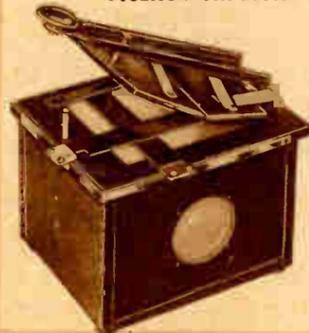
4x5" Size. A new method of making the actual exposure permits the use of this unit as both a printer and a safe-light. Safelight is always on. Accommodates all negatives from 35mm to 4x5". Positive paper alignment assured by metal guides set for accurate 3/16" margins. Masking bands fully adjustable. Double hinged sponge rubber covered pressure back. Hinged top all-steel and brass construction. Size: 7x7x9 1/2". Less bulb. Shpg. wt. 5 lbs.
