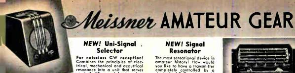
resonance into a unit that serves as both filter and loudspeaker. Rejects static and electrical noises almost in their entirety. Actuated only by a sustained audio frequency as furnished by
