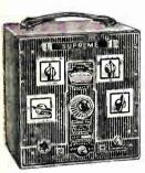
Produces six types of signals: (1) Straight C.W.; (2) 400 cy cle, 30 % standard audio modulated R.F.; (3) 400 cycles, 75% high level audio modulated dd R.F.; (4) Ex-ternal audio modulated R.F.; modulated R.F. (5) External frequency mod-ulated R.F.; (6) 400 cycle fixed audio note for testing audio amplifiers, etc.
