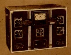
The HT-8 consists of a 25-watt transmitter and a receiver housed in a single cabinet that can be mounted on
