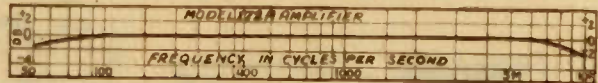
The above curve illustrates the remarkable frequency response of this amplifier as measured into the 500 ohm line.
