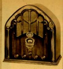
LAPAYETTE MANTEL 10 TUBE DUAL WAVE RECEIVER for 110 volt 50-60 cycle A.C. Tubes Used; 3-27s, 3-35s, 1-24A, 2-47s, 1-180. Complete with RCA TUBES. 2Y22088-Code (Marco). \$4150
