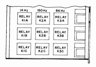
FIGURE 5-5 3D RELAY CHASSIS, REAR VIEW
