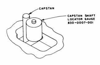
FIGURE 5-7 CAPSTAN SHAFT ALIGNMENT
