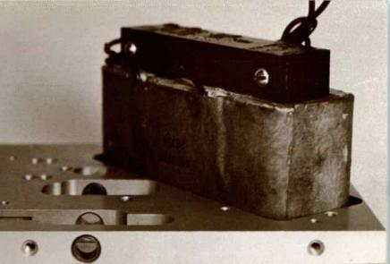
Half-inch thick, milled aluminum deck provides the massive support and stability needed to withstand shock and vibration and permit precision performance of all components.
