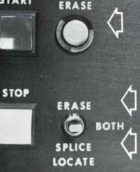
Erase indicator lamp reflects relative in-tensity of magnetic field during erasing process. Dims and goes out as erasure is completed.
