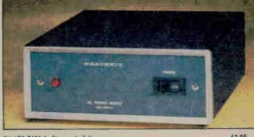
VFA-7401-1 SPECIFICATIONS: Output Voltage: 13.8 VDC regulated (Adjustable from approximately 12 to 15 VOC). Output Current: 4.0 amperes for 20 minutes (40% duty cycle). 3.0 amperes continuous. Output Regulation: Better than 1.5% from no load to full load (3.0 amperes). Output Ripple: Less than 2 mV peak-to-peak. Power Requirement: 120 VAC or 240 VAC, 50 60 Hz at 85 watts (juil load). Overall Dimensions: 3%," H x 74,4" W &
