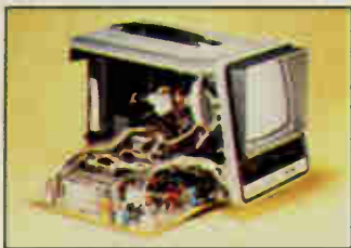
Pre-aligned modular circuit boards reduce assembly time and effort
