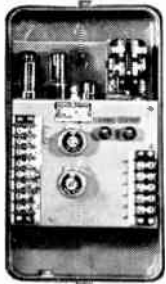
CR7505-N210G2 Photoelectric Relay (Cover Removed)
