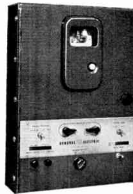
Automatic Inductrol with separately mounted control panel
