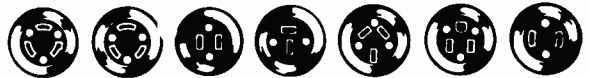
"K" Type Tandem "T" Type "Y" Type Crowfoot "U" Type Blade "X" Type
