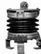
Model No. 9LA1H46 Thyrite arrester (one pole only) Max. rated 3kv for 4160-v grounded- or 2400-v ungrounded-neutral systems (half-unit shown)
