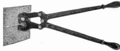
No. 6 For Punching \frac{1}{4} -In. Hole Through \frac{3}{16} -In. Iron
