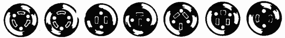
"K" Type Tandem "T" Type "Y" Type Crowfoot "U" Type Blade "XX" Type
