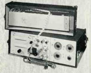
Battery pack plugs in back of amplifier which will always operate on A. C. until A. C. is interrupted—then change-over is automatic to batteries. Battery case section may be placed to the side or rear and need not be on top as illustrated above.
