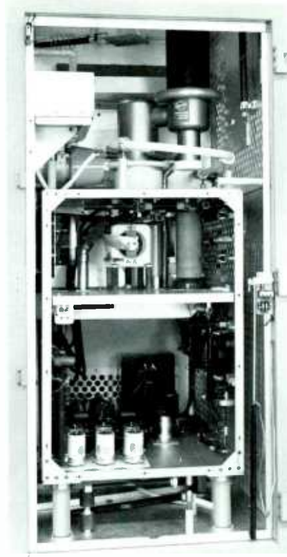
Rear view of RF isolation box showing power amplifier tube assembly and vapor phase cooling boiler.
