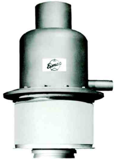
High power tetrode, 4CV50,000E, used in both the RF amplifier and modulator. Weighs only 35 pounds, and can easily be handled by one man.
