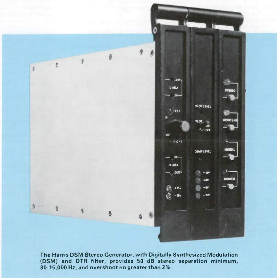
The Harris DSM Stereo Generator, with Digitally Synthesized Modulation (DSM) and DTR filter, provides 50 dB stereo separation minimum, 30-15,000 Hz, and overshoot no greater than 2%.
