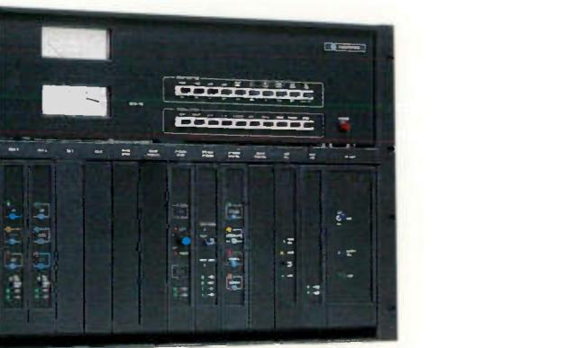
overshoot on any program material to 2% or less. As a result, 2 to 6 dB increased loudness can be achieved with no degradation of audio quality. Controlled transient response, high stereo separation, low crosstalk and low intermodulation distortion are all maintained with the increased loudness. The DTR filter can be switched off for stations whose formats do not require maximum modulation density.
