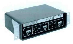
The Stanton 310B preamp features universal mounting by special brackets, instant selection of flat or NAB post-emphasis curves, switchable effective rumble filter, individual adjustment of gains and high frequency responses, trimming of the capacitive cartridge loading at the input and immunity to external magnetic AC fields.
