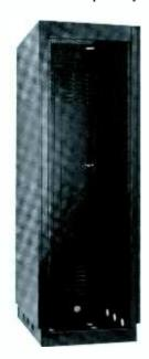
need, depending on stand alone or ganged installation. The cabinet is constructed of rugged 14 gauge C.R.S., equipment mounting rails are 12 gauge drilled and 10-32 tapped. Side panels are constructed of 18 gauge C.R.S. Thirty-seven rack units of mounting space are provided. Ventilation is provided by louvers in the cabinet top and in rear door. Prepunched holes for wiring access.
