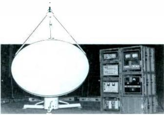
The S-2 "Flyaway" uplink system is the world's premiere high performance, totally "man-portable" C- and Ku-band uplink system. The entire system is packaged in 18 heavy duty aluminum/composite equipment cases, each of which conforms to international baggage size restrictions. The 2.4 meter Vertex antenna in the S-2 has a transmit gain of 49.0 dB and meets or exceeds the 29-25 FCC 2° spacing curves.
