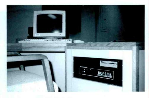
Printed logs from Digilink will automatically track actual ON AIR play of commercials and network errors. With it's capacity to be easily changed at any time, even during playback, Digilink is the perfect solution for satellite automation systems.
