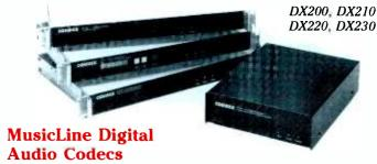
All MusicLine products have a built-in Inverse Multiplexer, (IMUX) which adds data capability of two, independent 56 or 64 KB/s channels so the codecs can be used on SW56, ISDN or dedicated digital lines. The IMUX may be disabled for use on T1, satellite channels or wireless modems. The encoders may be user-configured for stereo or mono operation.
