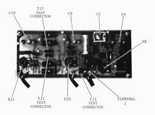
Figure 5-4. Directional Coupler 2Al Adjustment Locations
