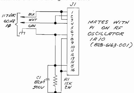
Figure 5-1. Oscillator Unit Bench Test Cable
