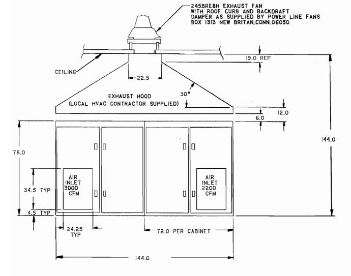
FIGURE 2-1. MW-50C3 OUTLINE DRAWING (SHEET 3 OF 4) 839 6587 128
