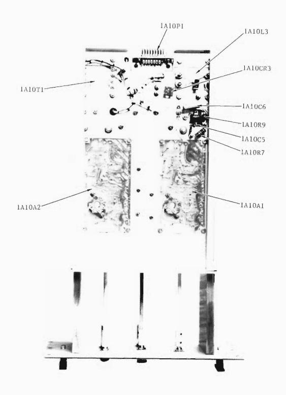
Figure 2-14. Oscillator Bottom
