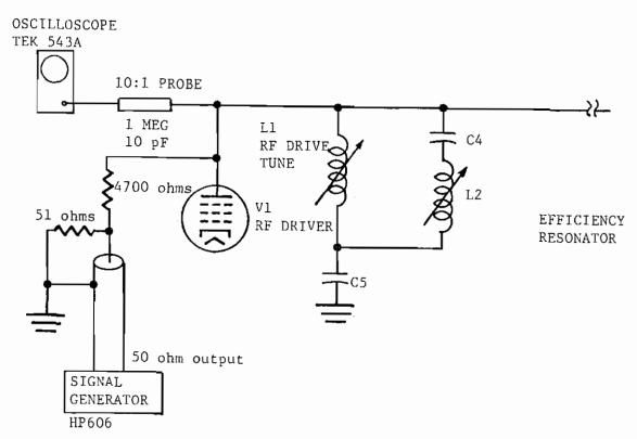
Figure 5-3. Test Setup for RF Driver Plate and PA Grid Efficiency Resonator Adjustment
