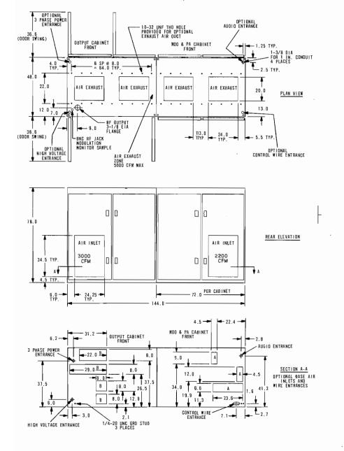
MECHANICAL DATA FOR MW-50C
