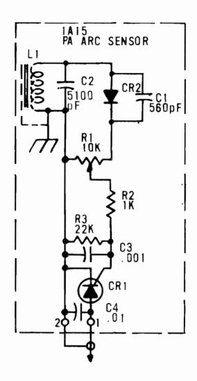
FIGURE 9-9. PA ARC DETECTOR 815 5021 001-B
