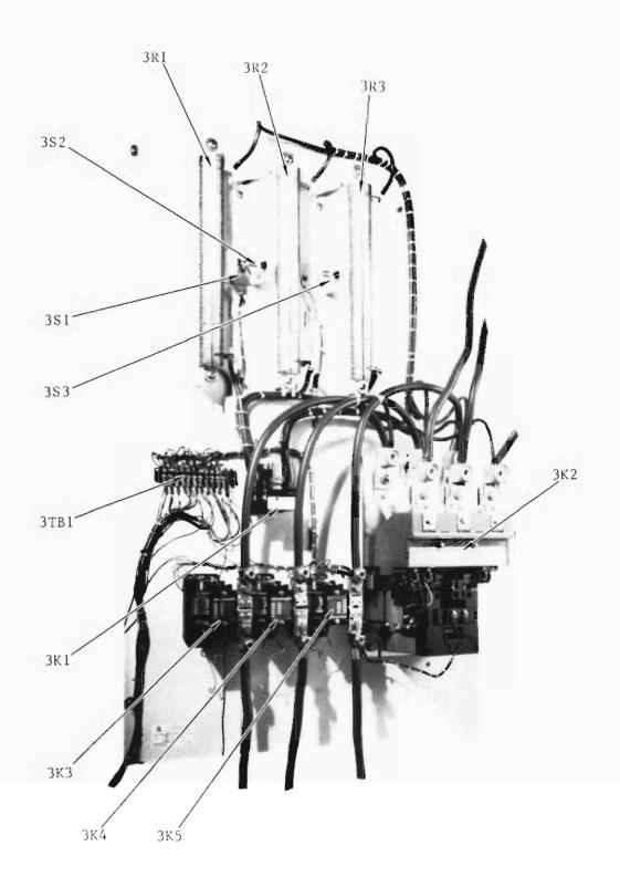
Figure 2-16. High-Voltage Step-Start Assembly
