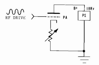
Figure 4-2. PDM Equivalent Circuit
