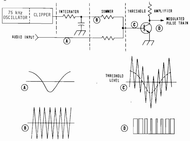
Figure 4-4. MW-50C3 Transmitter PDM
