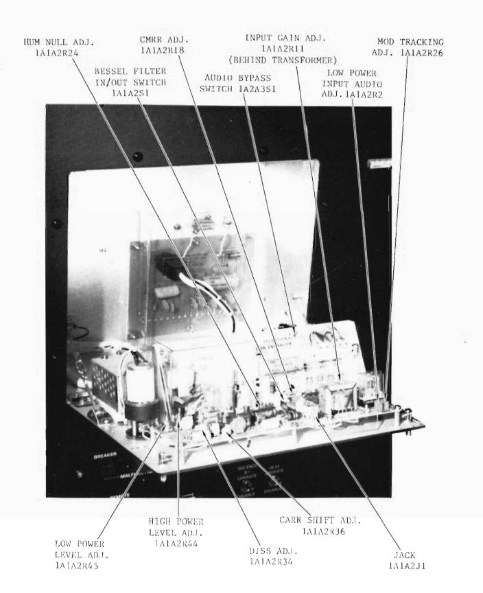
Figure 2-24. PDM Controls
