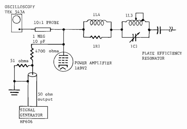
Figure 5-2. Test Setup for Efficiency Resonator Adjustment for PA Plate
