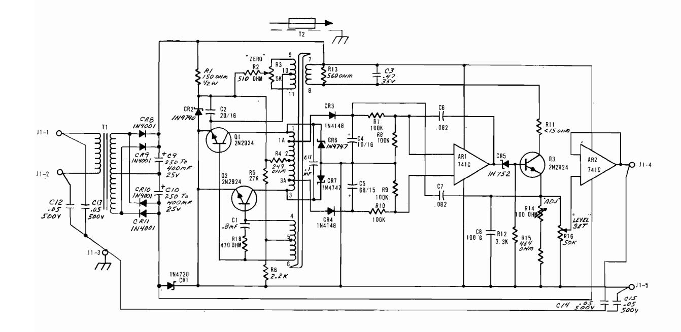
FIGURE 9-8. REMOTE PLATE CURRENT SENSOR 829 2756 001
