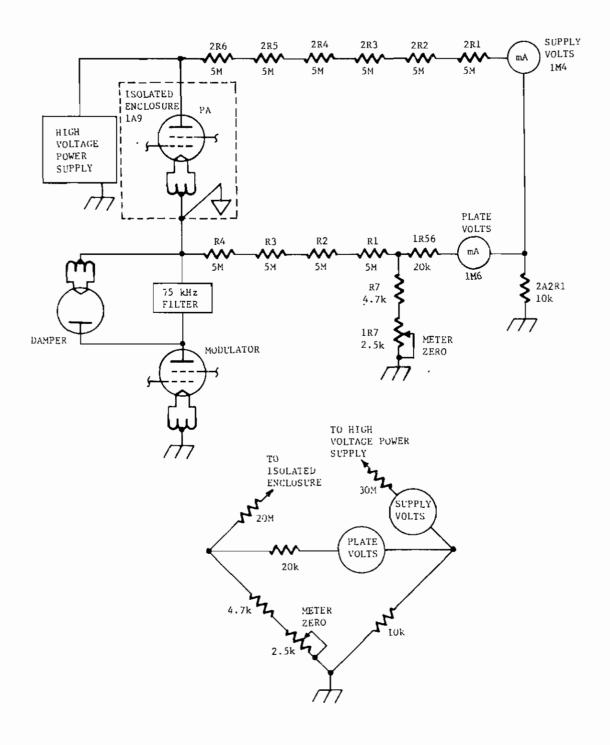
Figure 4-11. High Voltage Metering
