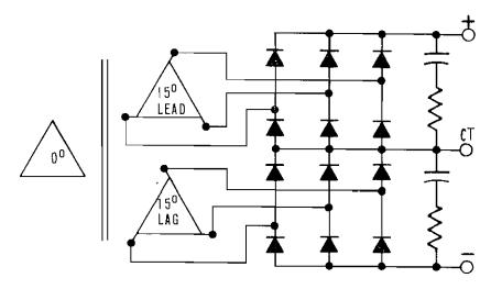
Figure 4-5. 12-Phase Circuit
