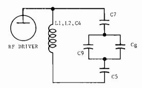
Figure 4-7. RF Driver Plate Circuit
