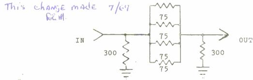
The 3 dB isolation network is contained in a  $1-5/8" \ge 2-1/4" \ge 2-3/4"$  aluminum box mounted inside the transmitter cabinet directly behind the TE-1 output connector.
