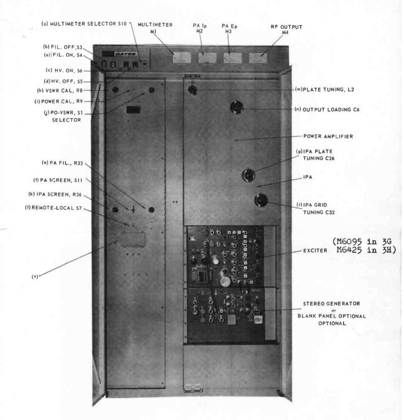
Figure 7.1 Front View, Showing Operating Controls
