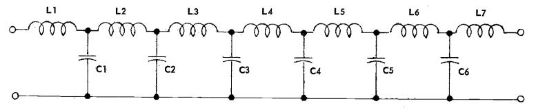
EQUIVALENT CIRCUIT - LOW PASS FILTER
