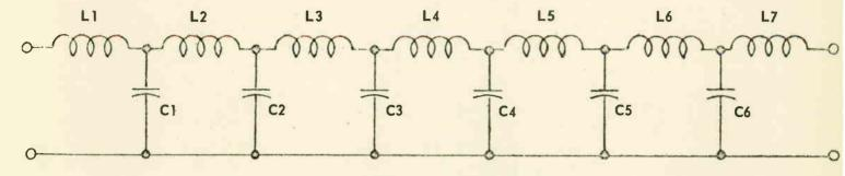
EQUIVALENT CIRCUIT - LOW PASS FILTER
