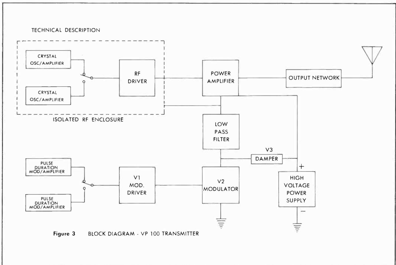
The modulator, V2, is connected through a low pass filter to the cathode of the power amplifier. The low pass filter provides the necessary function of removing the 70 kHz frequency component and the harmonics thereof and of recovering the audio as a modulating signal for the power amplifier. Note that the modulator is in series with the power amplifier.
