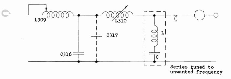
The condenser C can be the same type and capacity as at C316/C317. The circuit is tuned to normal loading on the fundamental without L. The coil L is tuned to the unwanted frequency when connected in parallel to C, using a grid dip meter. The coil L should be of 1/4" or 5/16" copper tubing. The mounting should be for minimum coupling to other circuit elements. With careful adjustment 20 to 30 DB attenuation may be obtained.
