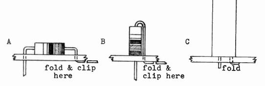
Fold the leads on the new part to the same spacing (A) & (B) as the mounting holes. Insert the part and fold the leads under the chassis to hold the part tightly against the top of the chassis. Clip off the excess wire.
