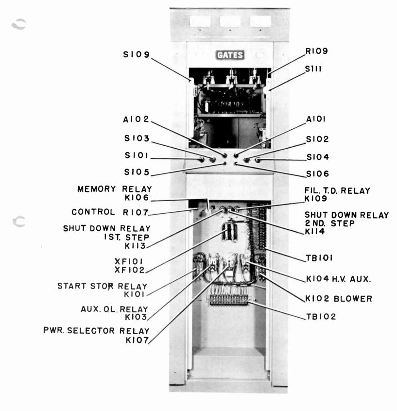
FRONT VIEW POWER CUBICLE BC5P/BCIOP The a.c. overload relays are of the instantaneous type. The tripping value is set by rotating the armature on the threaded shaft; a tab aligns with narkers on the armature to indicate the tripping current. The armature is locked in position by a locknut. This should be tight so that the relay holds calibration.
