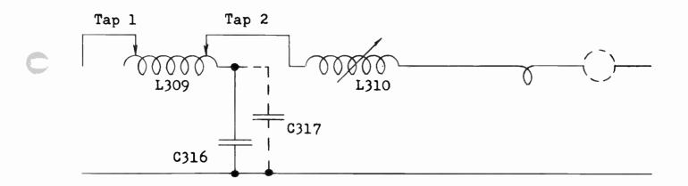
Tap 2 is adjusted so that the inductance between this tap and the end of the coil connecting to the coupling condensers, with the coupling condensers C316/317 form a series resonance circuit at the unwanted frequency. The position of tap 2 may be critical to 1/4". The normal loading is then adjusted by the position of tap 1. This circuit shows 10 to 20 DB attenuation to the undesired signal.
