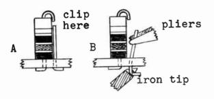
place iron on fillet and push wire through the hole until the hook can be clipped off.
