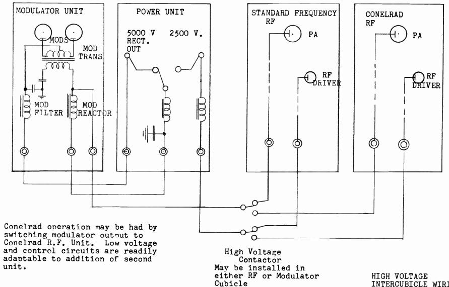
HIGH VOLTAGE INTERCUBICLE WIRING FOR ADDITION OF CONELRAD R.F. UNIT
