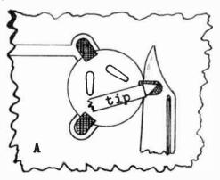
Place the iron tip on top of the folded over mounting ear. As the solder melts, slip a thin knife between the mounting ear and the copper conductor pad. DO NOT PRY THE TAB UP WITH THE KNIFE! See (4-B) for bending ears away from chassis. When the knife is completely under the ear, remove iron and let the solder cool.
