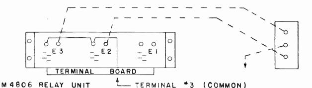
Solder two leads to A.C. relay terminals opposite common connection, and connect to two outside terminals of motor switch.
