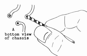
Use a small metal twist drill (1/8" dia. or less) to clear the <u>hole</u> <u>only</u> in the fillet of solder. Twirl the drill by hand. Do not attempt to remove all of the solder in one turn, do it slowly and carefully.
